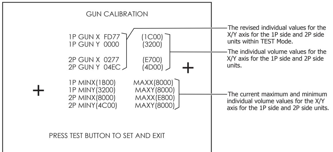
**FIG. 9-3c02 Calibration Screen**
