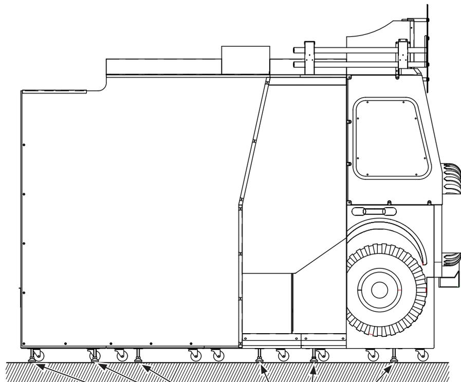
Ensure that all of the adjusters are in contact with the floor.
