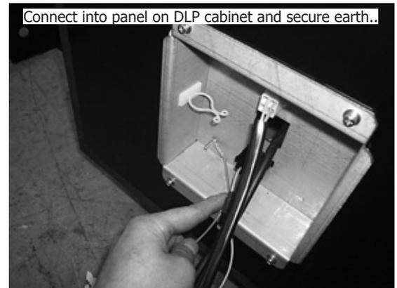
Connect into panel on DLP cabinet and secure earth..
